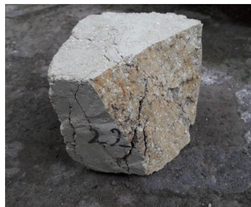
Figure 4 Sample Condition After Compressive Strength Test
