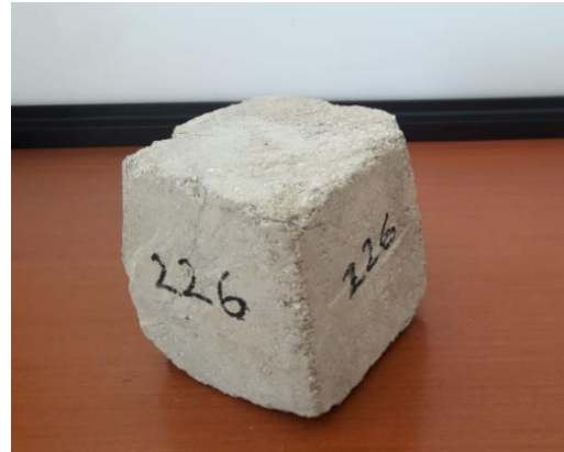
Figure 3 Samples of Rock Cut in Cube Shape
